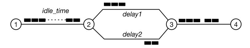
No packet reordering if idle\_time > | delay1 - delay2 |
