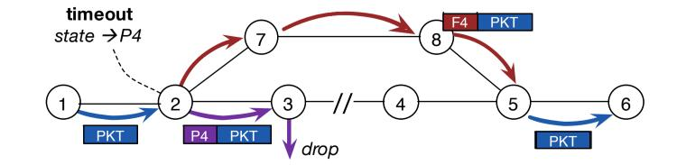
\* As long as packets are received from a given port, that port can be used to reliably transmit other packets. When no packets are received for a given interval, a node can request its neighbor to send an "heartbeat". If no reply is received within an interval, the port is declared down.
